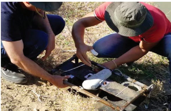
Figure 44: Preparing the SonTek-IQ for deployment in its custom-designed frame, October 2017 (Source:WMI)
